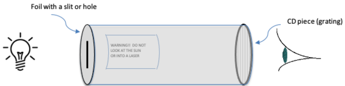
Figure 1.2 - The cardboard tube spectroscope. Look through the grating or CD piece on the back end of the tube toward the foil. This drawing shows a slit on the front end but you can also just poke a small hole into the center of the foil.
