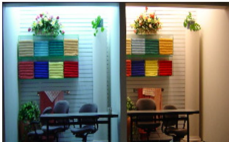
Figure 1.4. Photo taken at the Southern California Edison Lighting Center, 2004. The items in the displays are the same colors on both sides of the wall, only the lighting is different.
