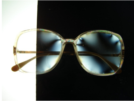
Figure 6.5 - Eyeglasses viewed between two crossed polarizers. The lenses are stressed by the frames.
