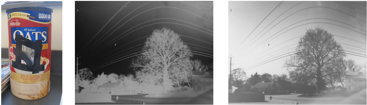
Figure 2.3. (Left) An oatmeal box pinhole camera. The pinhole is in the piece of aluminum taped to the box. (Middle) The film paper was taped inside the box, following the curve. The image on film paper is a negative. (Right) The image was scanned and digitally processed to form a positive image.
