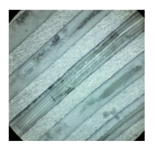
NCMR 1903-1938) During inspection of fiber noticed a bright spot. When examined under microscope, noticed that the section of fiber is missing coating
