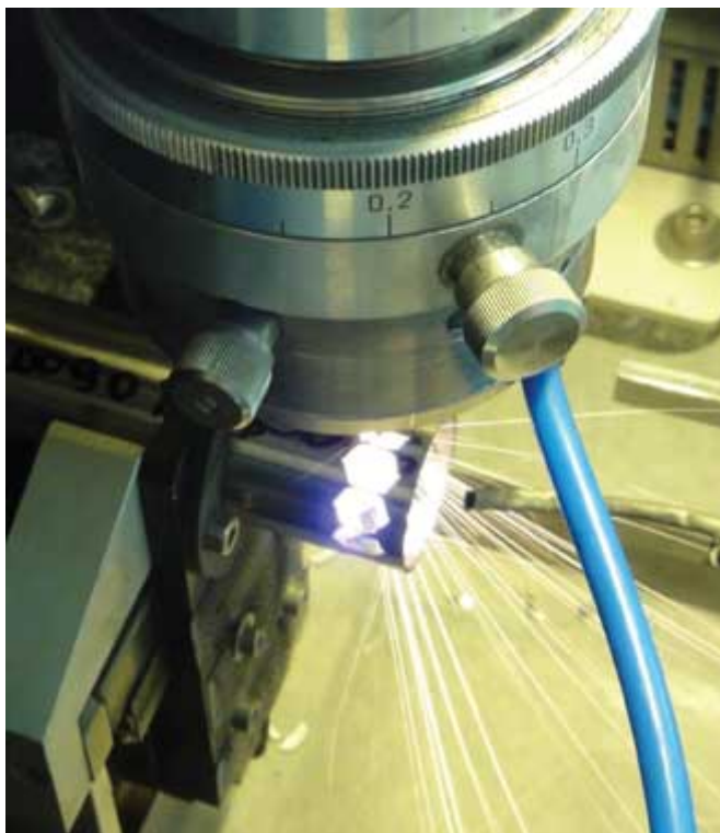
A fiber laser cuts a tube for a medical device.
