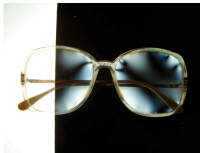
Figure 13 – These eyeglasses are resting on a light box covered with a sheet of polarizing film. A second piece of film oriented at right angles to the first is covering the eyeglasses on the right. Stresses in the glass lenses is apparent under the top polarizer.
