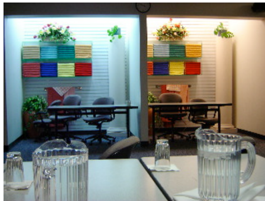
Figure 1 - The wavelength content of a light source influences the perceived color of objects. (Photo taken at the Southern California Edison Lighting Center, 2004.)
